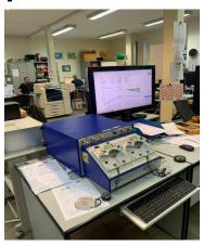
The Laboratory of Italiana Conduttori Srl, systematically completes a comprehensive and detailed analysis of the following characteristics: Construction, Weight, Physical Dimensions, Mechanical Strength, Electrical Resistance of conductors, Impedance, Capacitance, Attenuation Losses, and Structural Return Losses (SRL). In addition, thanks to the purchase of the new AESAVEGA analyzer we are able to measure all electrical characteristics of data transmission cables from cat 5e to 8 up to 4 Ghz.
