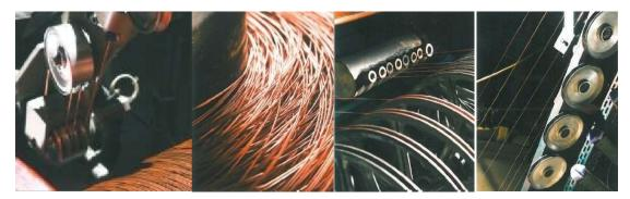
Description: red copper wires with a diameter between 0.31 mm and 3.40 mm are drawn.
