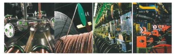
**Description**: cable shielding is formed on the primary insulation. It consists of a braid created using conductive wires, with or without interposed conductive ribbons. The company uses over 200 braiding machines, which offer great flexibility and a high production capacity.
